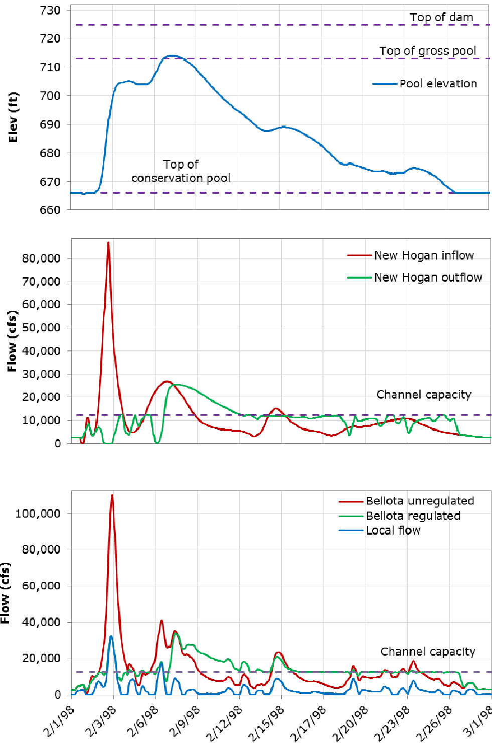
Figure 29. Reservoir routings of the 1998 event scaled using the New Hogan frequency curve to the p=0.005 3-day flow
