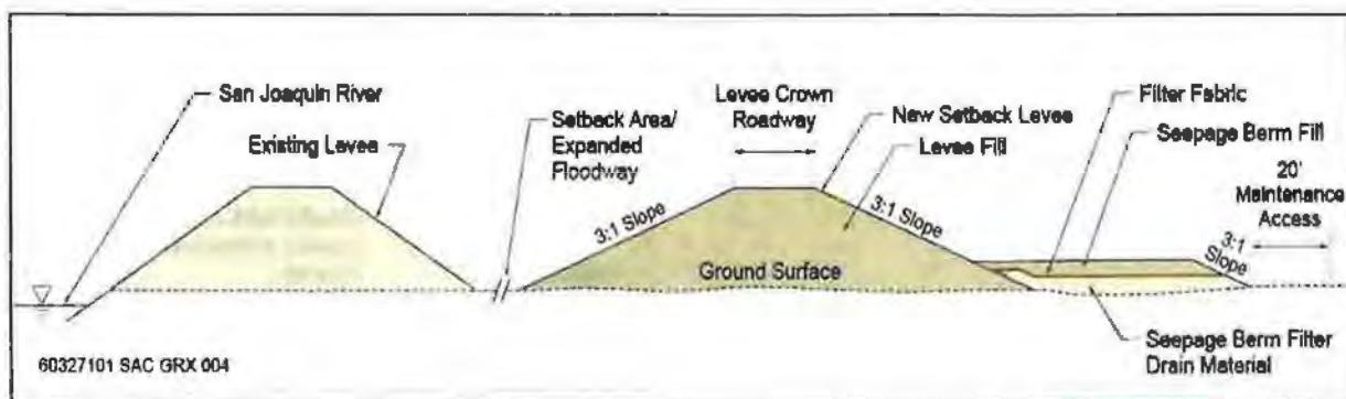
Figure 3f. Typical setback levee.
