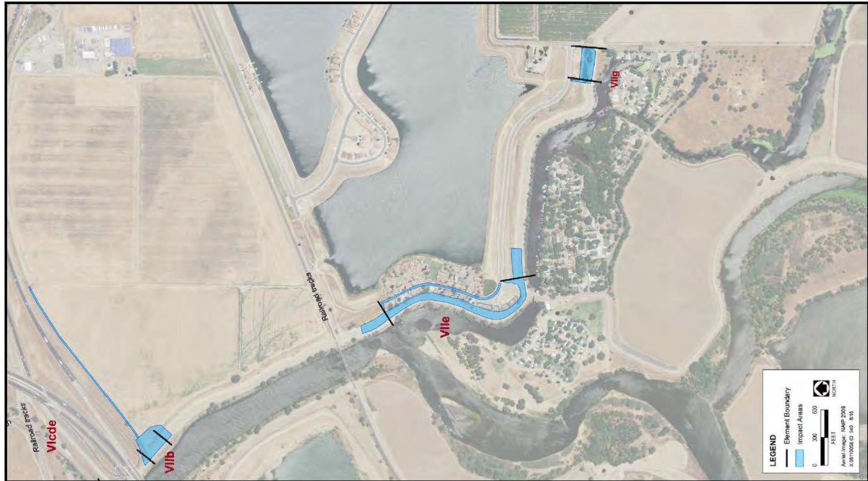
**Figure 4c:** Locations of Project Levee Construction Elements
