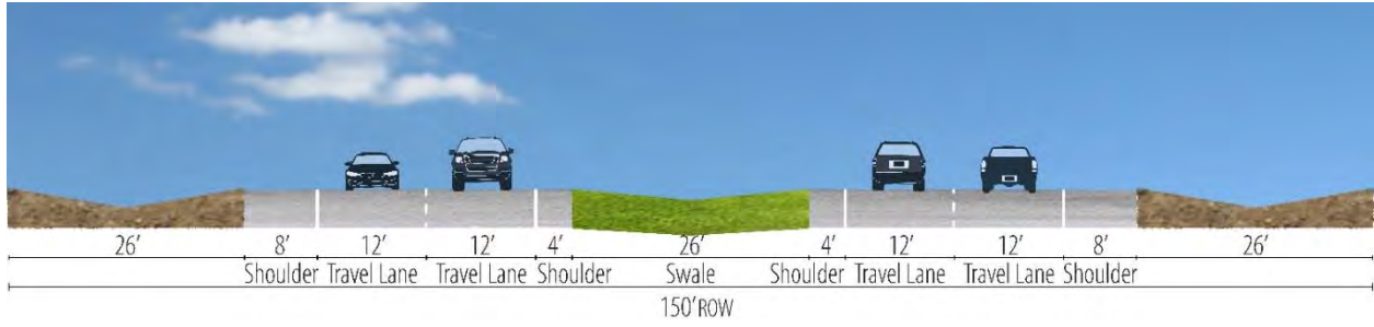
Figure 1. SR-193 typical cross section between 3000 West and West Davis Corridor.
