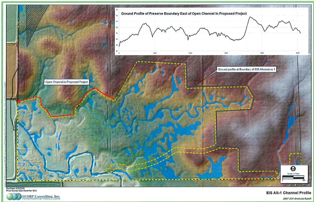
For 404(b)(1) Alt. 3 an additional approximately 7,000-ft of channel would also be required to follow the edge of the proposed development and not cross through the preserve area. The figure shown below (Modified 404(b)(1) Alternative-3 Channel Profile) includes a profile of the ground surface along the southern edge of the 404(b)(1) Alt. 3 (shown in gray on the figure) beginning at the point of connection with the originally proposed channel system (shown in red on the figure).
