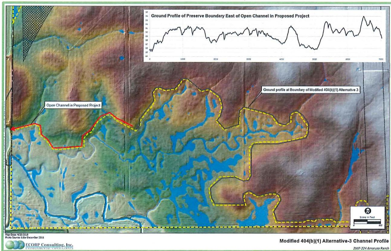
As can be seen on the surface profile, the elevations along either the EIS Alt 1 or the 404(b)(1) Alt. 3 boundary do not lend themselves to a gravity flow scenario due to a number of high and low points along the profile. Two options were considered for drainage for this alternative:
