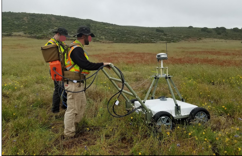
MetalMapper 2x2 being used to locate UXO. Image courtesy of Geometrics Inc.
