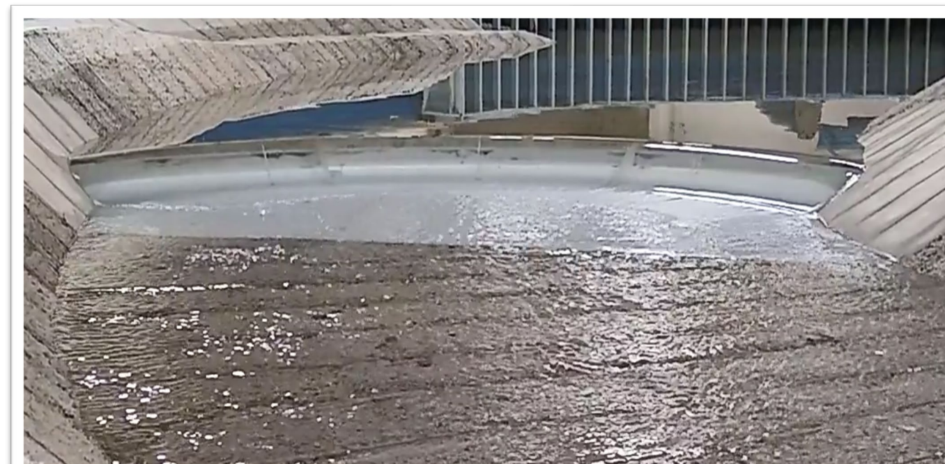
Spillway Model With Ogee Weir
