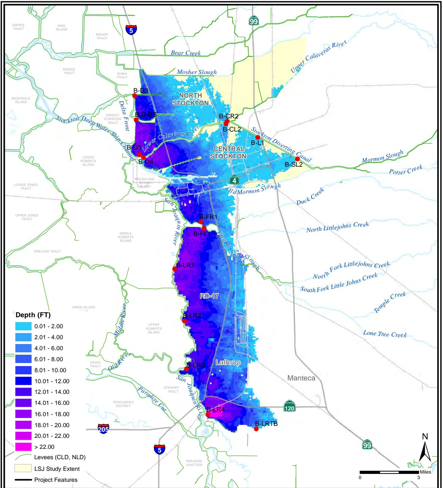
NOTE: Breach simulation shown if levee does not pass assurance criteria. 1) Assurance less than 90% the levee does not pass criteria 2) For assurance between 90 and 95% levee must have minimum of 3 feet of freeboard to pass criteria. 3) For assurance greater than 95% levee must have minimum of 2 feet of freeboard to pass criteria
