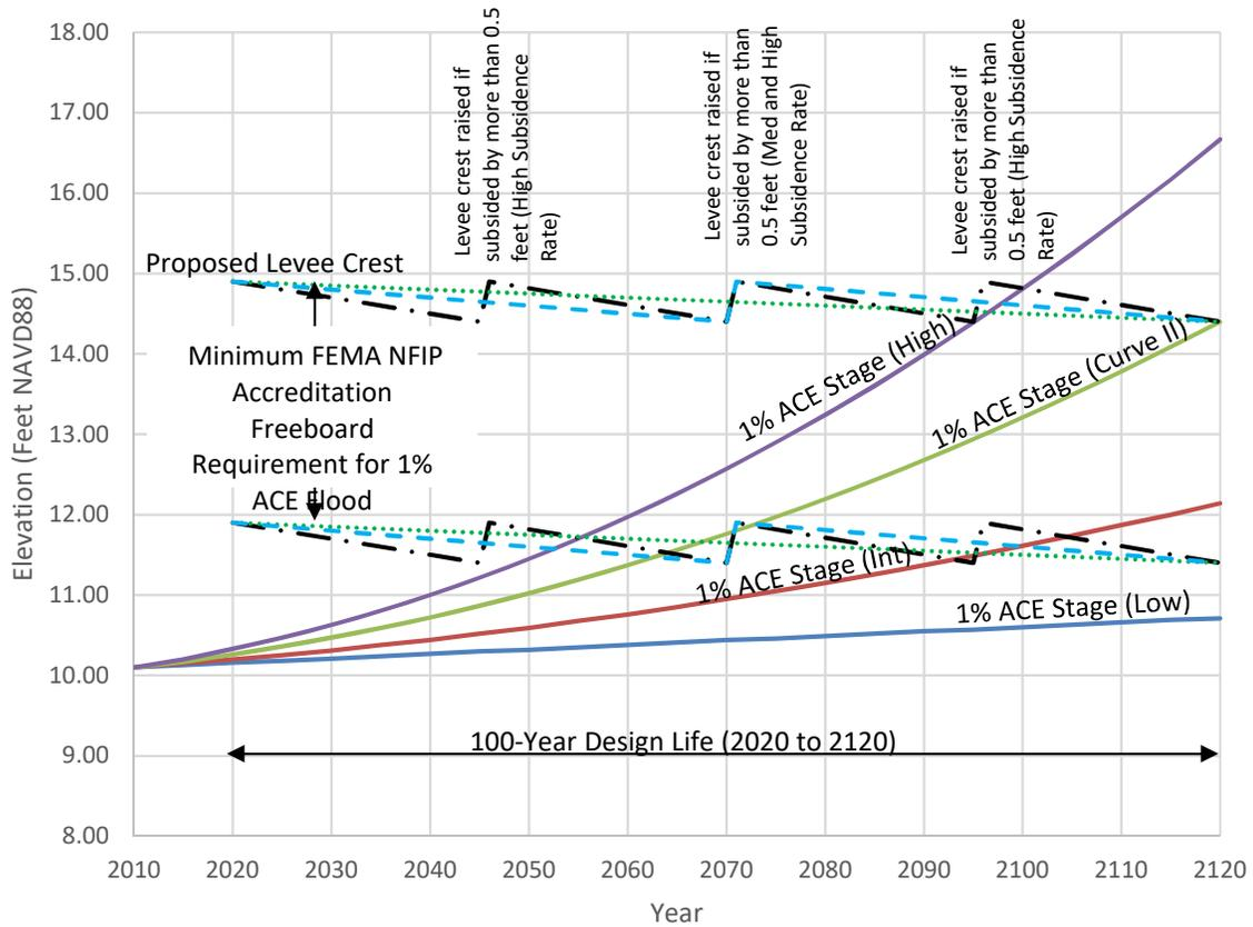
Year Water Surface Expected to Exceed Minimum Freeboard Requirement Assuming Levee Crest Restoration after 0.5 feet of subsidence is observed.
