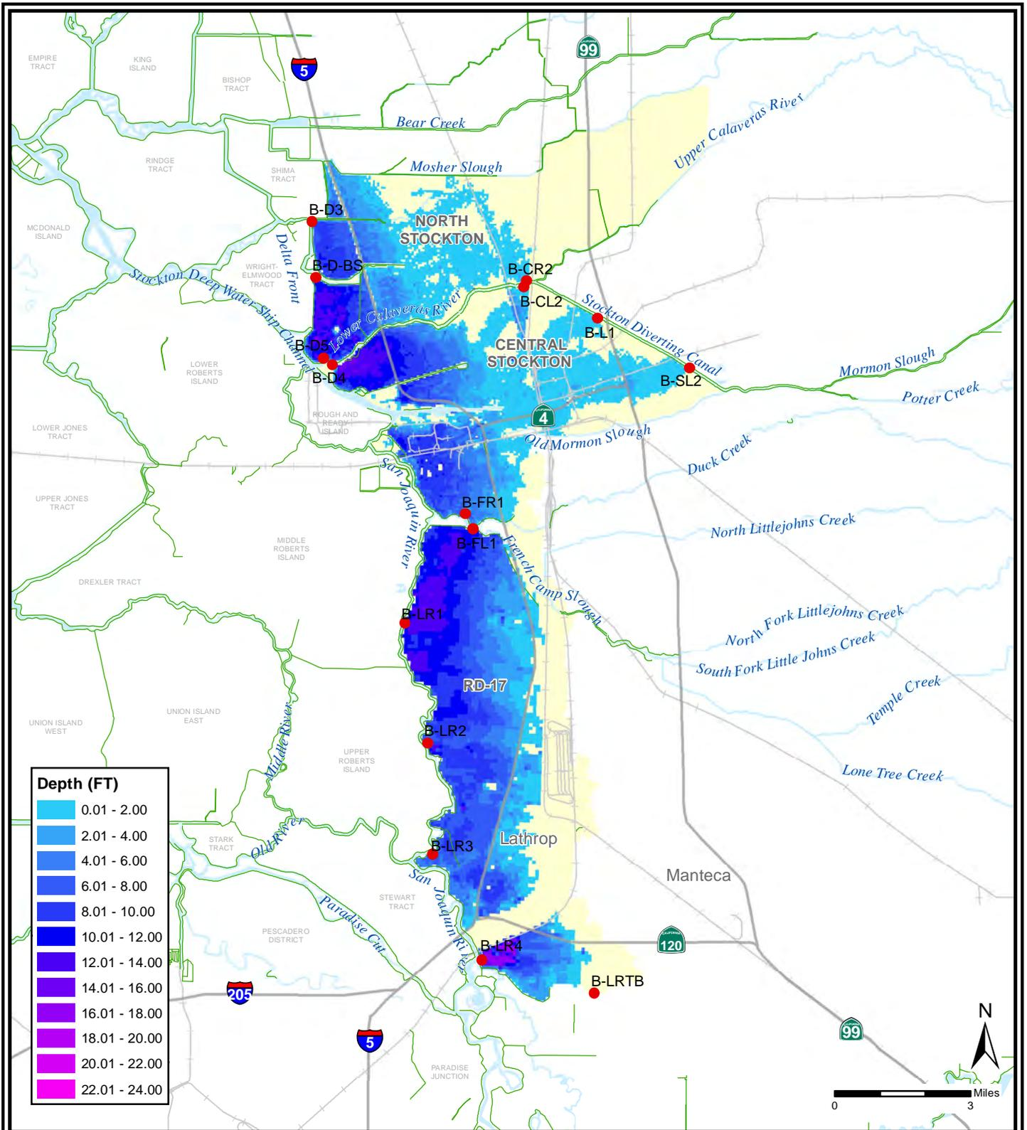
NOTE: Map intended to show the potential floodwater depth from a breach along any of the principle flood sources identified in this study. All breach simulations shown regardless of levee performance.
