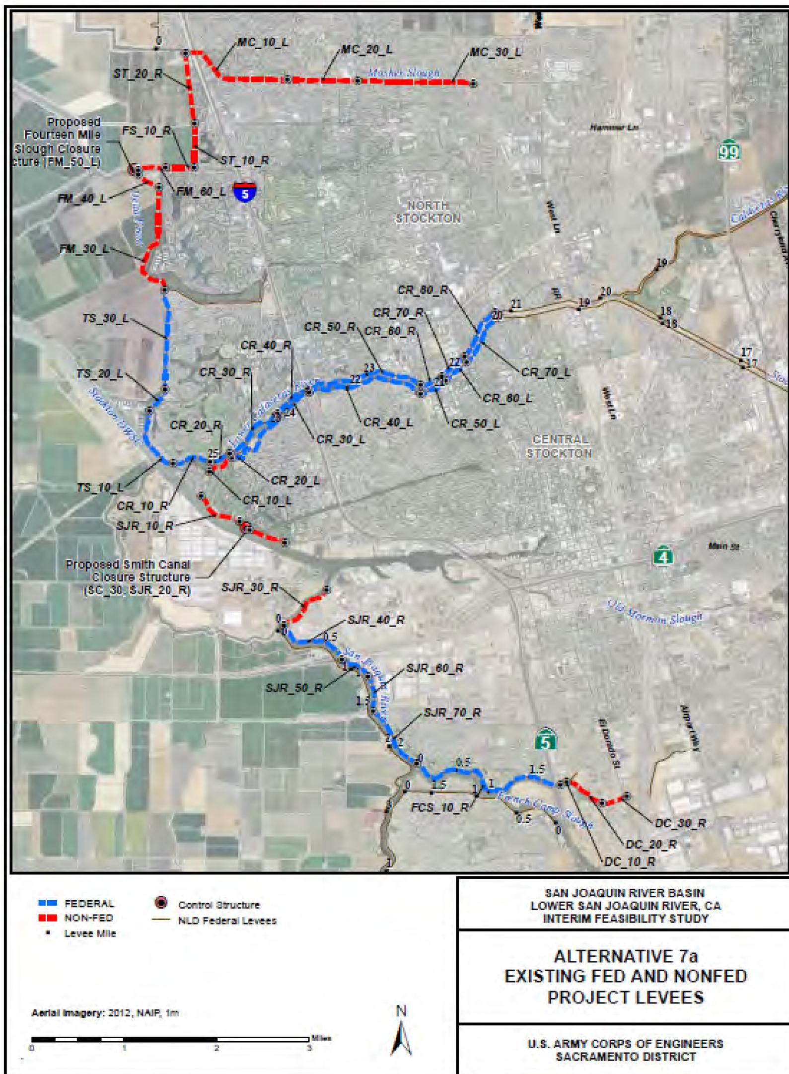
Figure 3. Federal and non-Federal levees included in the Recommended Plan
