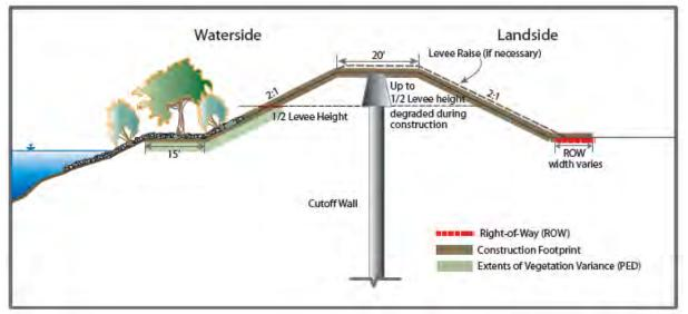
Figure 3. Fix-in-place with Cutoff Wall.
