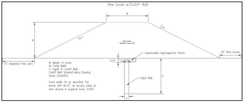
Figure 9. New Levee with Cutoff Wall Typical Plan
