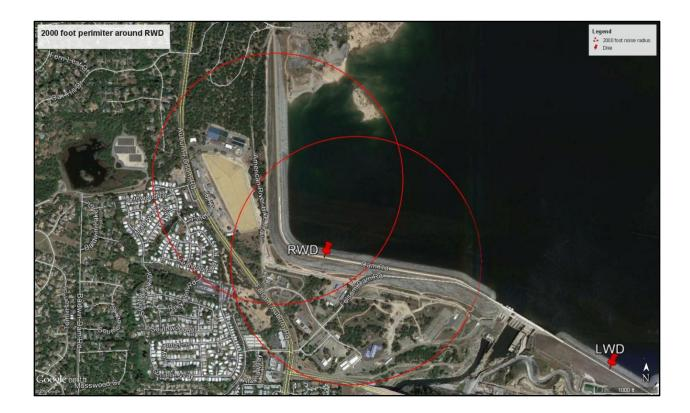
Figure 3-17. 2,000 Foot Noise Buffer around the Right Wing Dam. \*Two buffers were used in assessment due to size of the Right Wing Dam.
