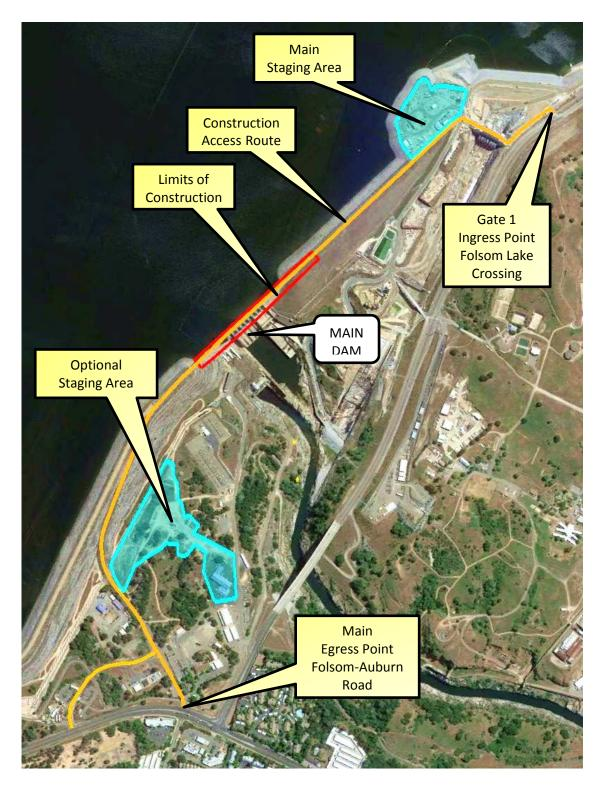
Figure 2-10. Main dam Tainter gate refinements: Limits of construction (red lines), construction staging areas (blue lines), and construction access route (orange lines).
