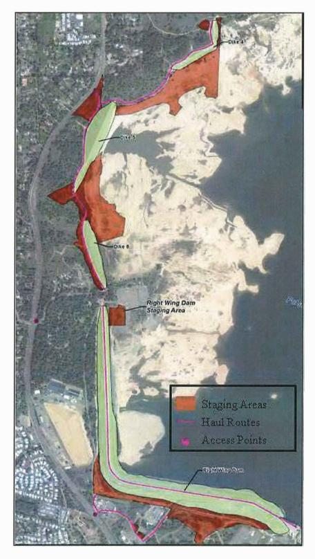
Figure 9. Staging areas, access points, and haul roads associated with Dikes 4, 5, and 6, as well as Right Wing Dam.
