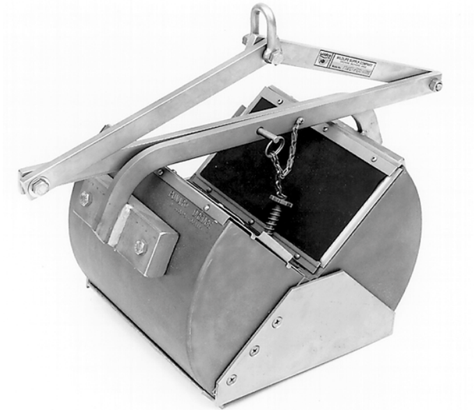
Figure 2 : Ponar (L) and Gravity Corer (R)
