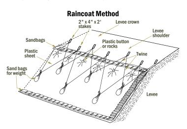
A tie-down button or small stone (preferably round) is secured through both layers of visquine. If a stone is used, tie a slip knot and double half-hitch to secure it. Fasten buttons to the visquine and tie off to the stakes using a minimum 250 lb. tensile strength twine with these points in mind:
