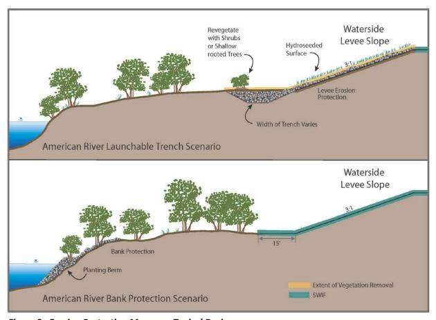
Figure 3. Erosion Protection Measures Typical Design.
