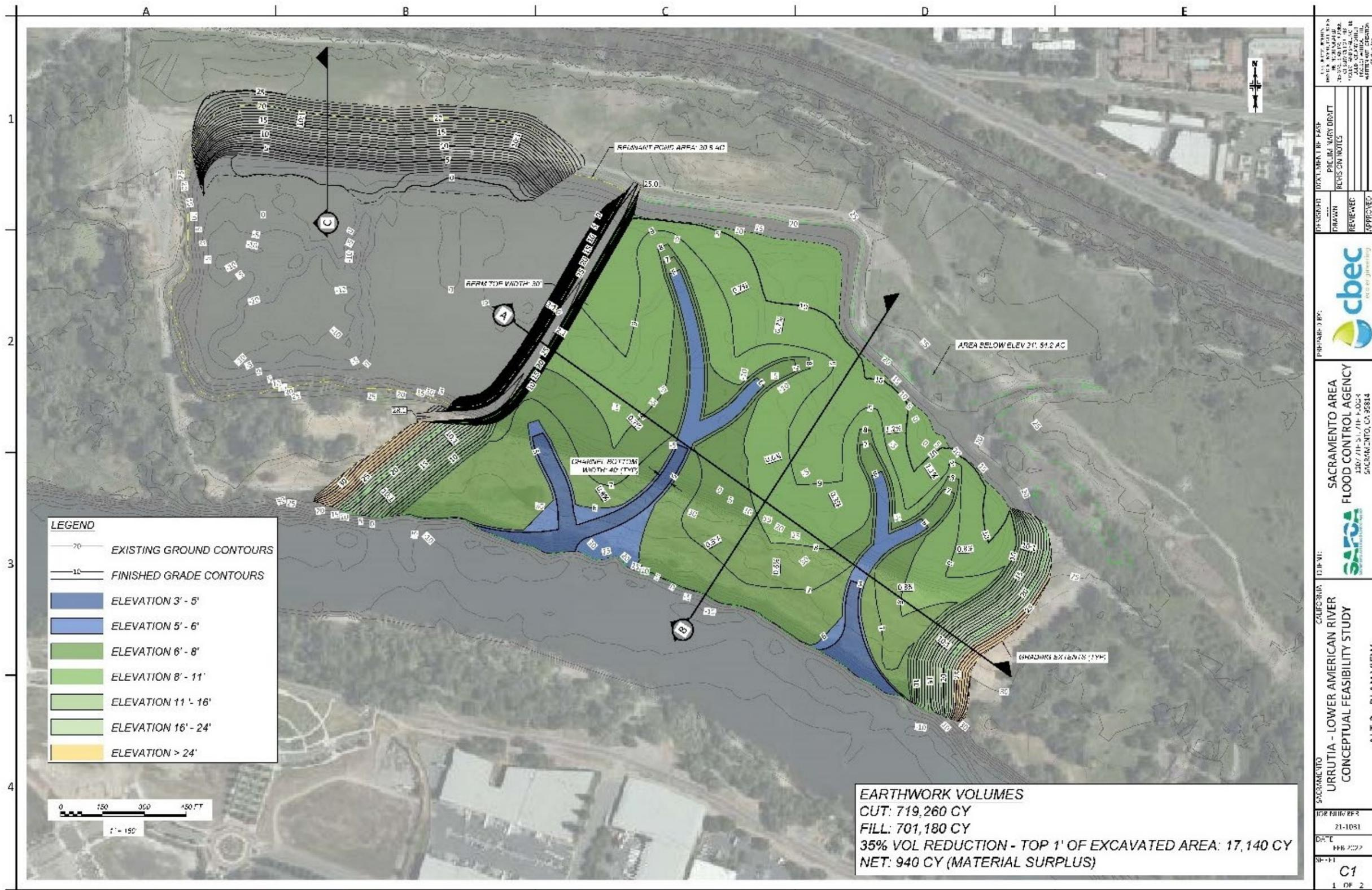
Figure 3.7.1-1. Conceptual Site Design with Pond for Alternative 4a
