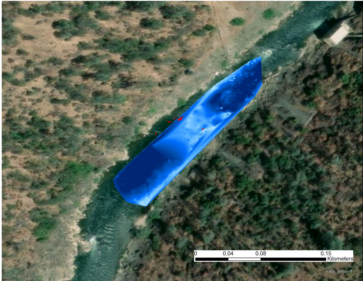
Figure 12. Mapped salmonid redds (pots and spill) in injection vicinity in the study area of the lower Yuba River below Englebright Dam, CA from September 16, 2024 to April 28, 2025. Blue shading indicates gravel elevation from post-injection gravel mapping in fall 2024.
