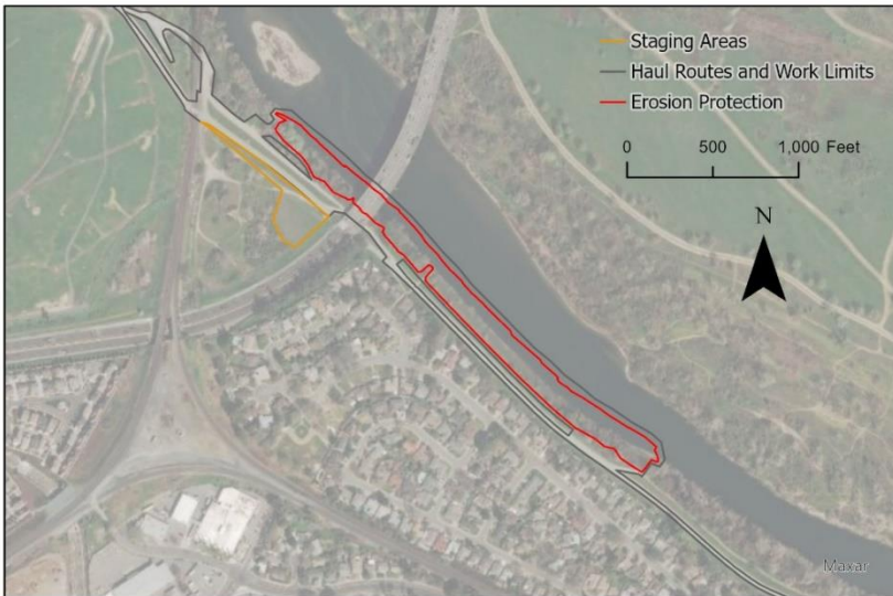
Figure 1- 4 Bank Protection and Launchable Toe Footprint
