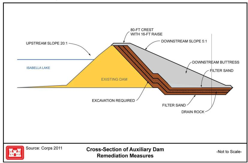
Figure 2-4-FEIS Cross-Section of Auxiliary Dam Remediation Measures
