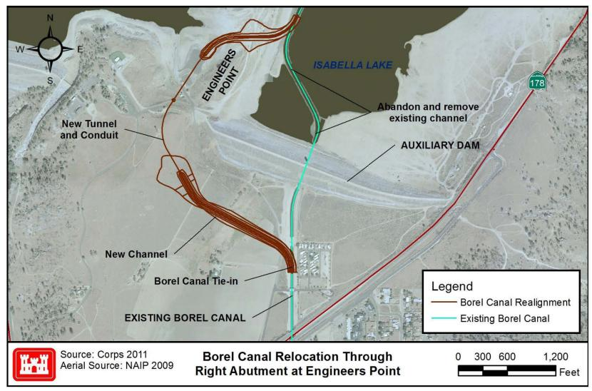
Figure 7 Preferred Alternative – Borel Canal Relocation
