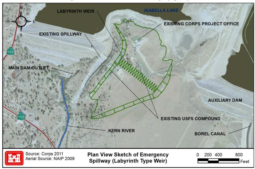
Figure 5 Preferred Alternative – Emergency Spillway
