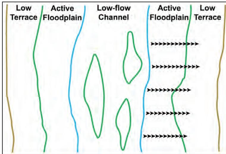
**Figure 34. Step 5 of the field verification procedure. The arrows indicate potential foot paths along which changes in percent vegetation cover by strata, stand age, species composition, and dominant sediment textures associated with the active floodplain/low terrace transition should be observed and recorded.**
