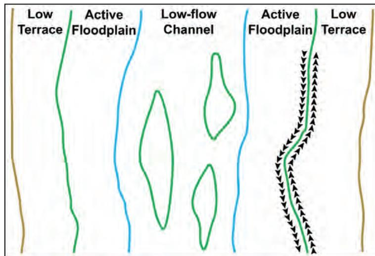
**Figure 35. Step 6 of the field verification procedure. The arrows indicate foot paths that should be followed to verify that the transition from the active floodplain to the low terrace identified through observing changes in vegetation, sediment texture, and possibly a break in slope is reliable in both the upstream and downstream directions.**
