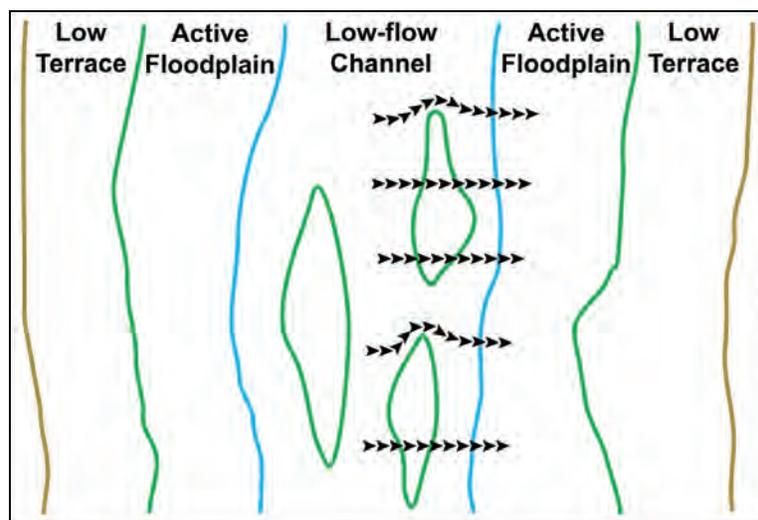
Figure 32. Step 3 of the field verification procedure. The arrows indicate potential foot paths along which changes in percent vegetation cover by strata, stand age, species composition, and dominant sediment textures associated with the low-flow/active floodplain transition should be observed and recorded.
