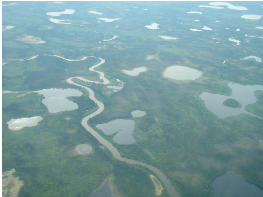
Figure 73. Abundant wetlands in the Alaskan interior, despite relatively low annual precipitation, reflect the presence of permafrost, which impedes infiltration and drainage.
