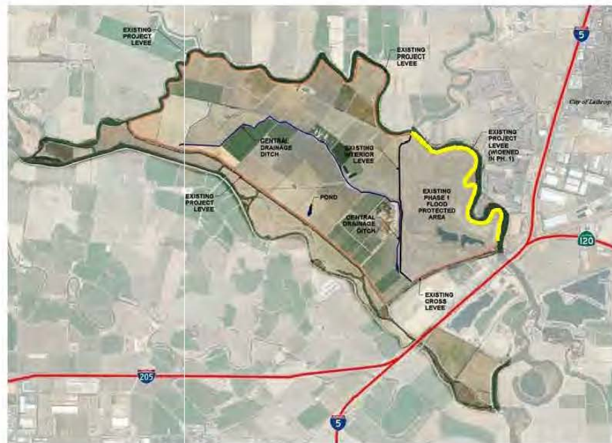
Figure 1. Features of existing scenario (courtesy MBK Engineers)
