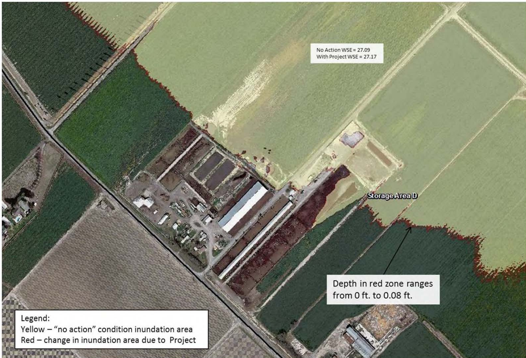
Figure I-14. Detail of Storage Area D and E 200-year inundation, No Action and With Project (1 of 1)
