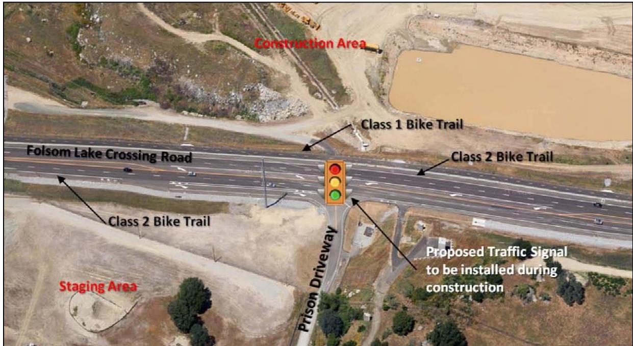
Figure 5. Temporary Traffic Signal Location.
