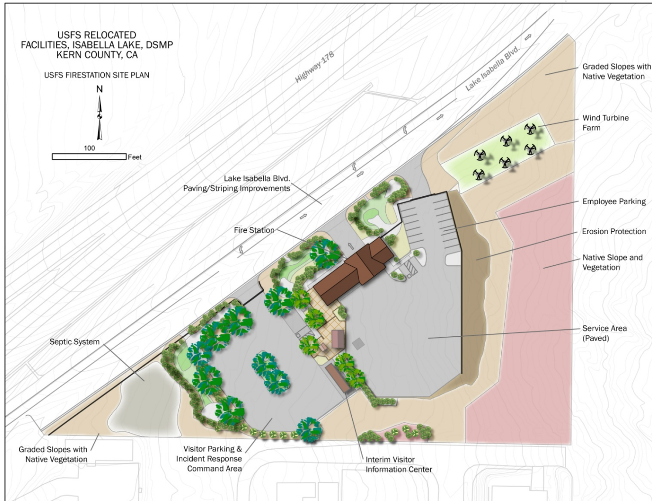
Figure 6. USFS Fire Station Response Center Concept Design.
