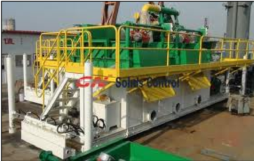
Photograph 2. Slurry Mixing Hopper Pit
